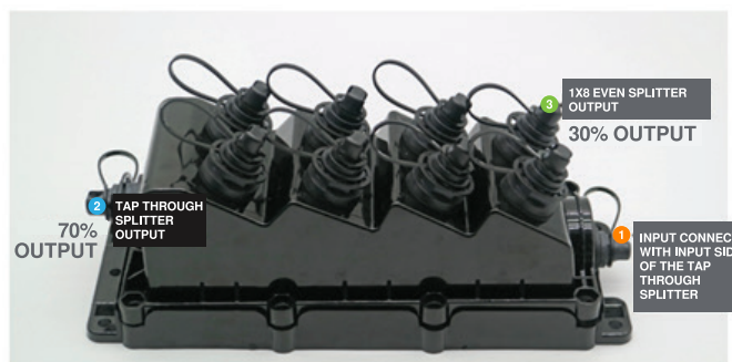
Unterminated 8-port LB-MST 1x2 70/30 coupler with 1x8 splitter (LB-MST-108-70/30)
